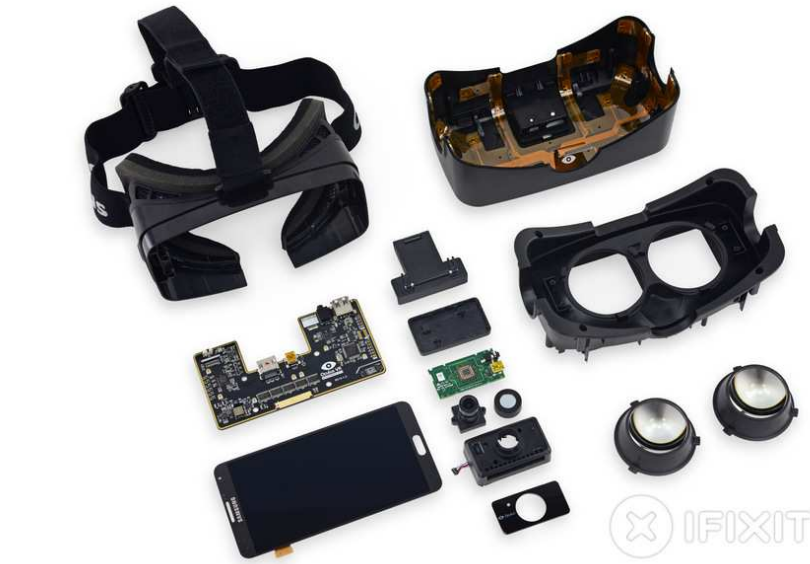
Figure 2.12: Disassembly of the Oculus Rift DK2 headset (figure from www.ifixit.com ).
