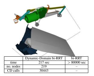
Fig. 9. An example from the manufacturing industry. The goal is to find a collision free path dismounting a wiper motor from a car body.
