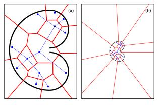
Fig. 1. A bug trap problem in high dimensions can be a challenging problem for RRT-based planner (a). It becomes much more challenging when a region for sampling is enlarged (b). The tree constructed by the RRT planner is shown in blue (black nodes and edges) and the Voronoi regions associated with the nodes of the tree are shown in red (gray edges).
