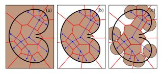
Fig. 3. For a set of points inside a bug trap different sampling domains are shown: (a) regular RRTs sampling domain, (b) visibility region, (c) dynamic domain.
