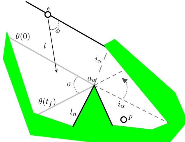
**Fig. 6.** Pushing a gap. The evader travels on  $l$  at angle  $\phi$  as to maximize the angle  $\sigma$ , thus maximizing contamination. As the evader moves, the gap moves with it, and so does the gap extension ray  $i_\alpha$ . In the extreme case,  $i_\alpha$  coincides with  $i_n$ . If the pursuer crosses  $i_\alpha$ , the evader is detected.
