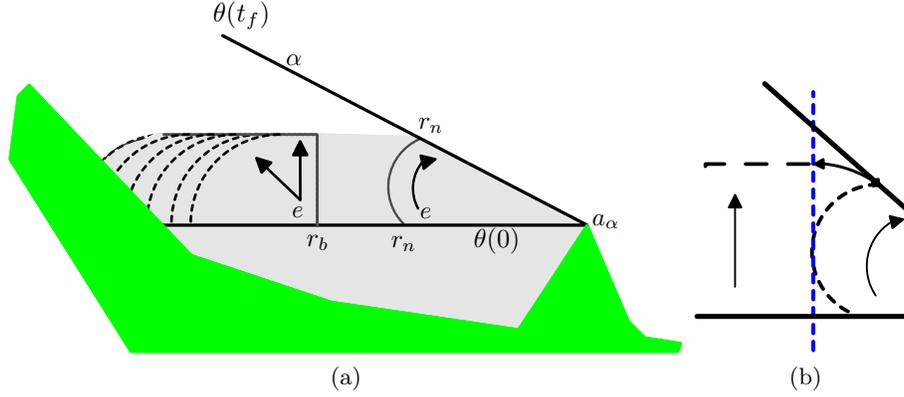
**Fig. 2.** Recontamination fan. (a) Gap  $\alpha$  moved from  $\theta(0)$  to  $\theta(t_f)$ . Any evader before  $r_n$  follows exactly the angular motion of  $\alpha$ . Any evader after  $r_b$  can be anywhere inside a circular section of radius  $v_e t_f$ . The net effect is a line segment sweeping perpendicularly to the original position. (b) For  $w(t)$  constant, the contamination region between the vertical dashed line and the dashed arc is bounded by the involute of a circle.
