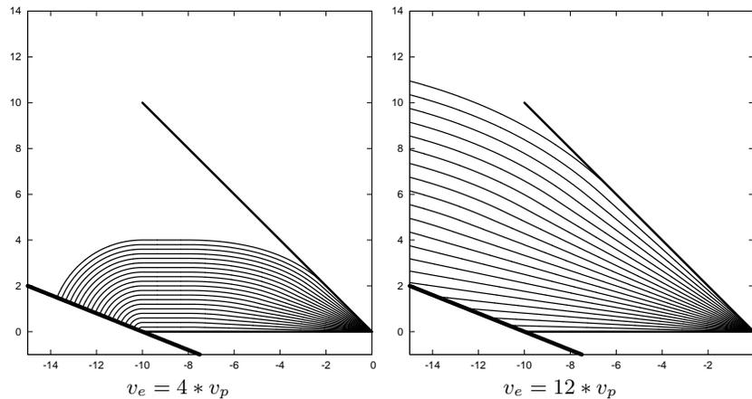
**Fig. 4.** Computed example of a recontamination fan for a pursuer linear motion. The gap start at  $\theta(0) = 0^\circ$ , and ends at  $\theta(1) = 45^\circ$ . The thick line on the bottom-right represents an edge of  $\mathcal{R}$ . The evolution of the contamination is shown for times between  $[0, 1]$ .
