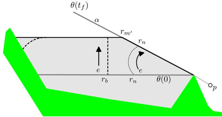
**Fig. 3.** Piecewise-linear approximation. Instead of computing the exact contamination boundary, an approximation is easily generated by ignoring the angular velocity of the gap, considering only its final angular position.
