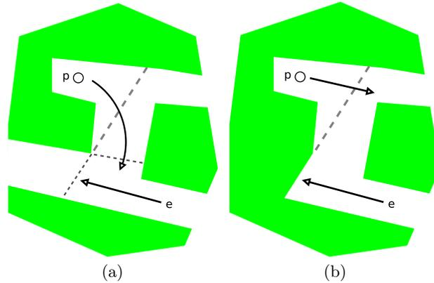
**Fig. 7.** Clearing equivalent polygons. The pursuer considers the gap extension ray in (a) as the actual inflection ray. This is equivalent to clearing the polygon in (b).
