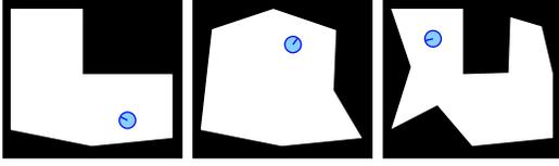
Fig. 2. When the environment is uncertain, the identity of the environment becomes part of the state of the system. Above are three states for an example system containing a mobile robot in the plane with environment uncertainty.
