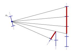
Fig. 4. Computing the set  $V_i$  of cells visible from a cell  $s_i$ . The diagram depicts three cells fully visible from the midpoint of  $s_i$  and one cell that, because of an obstruction, is only partially visible. All four cells are included in  $V_i$ .
