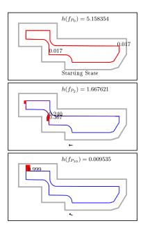
Fig. 8. Localization in a simple environment. [top] The initial probability distribution around the environment boundary. [middle] An intermediate step resulting from the first two steps of the plan. [bottom] The resulting distribution after the localization plan is run.
